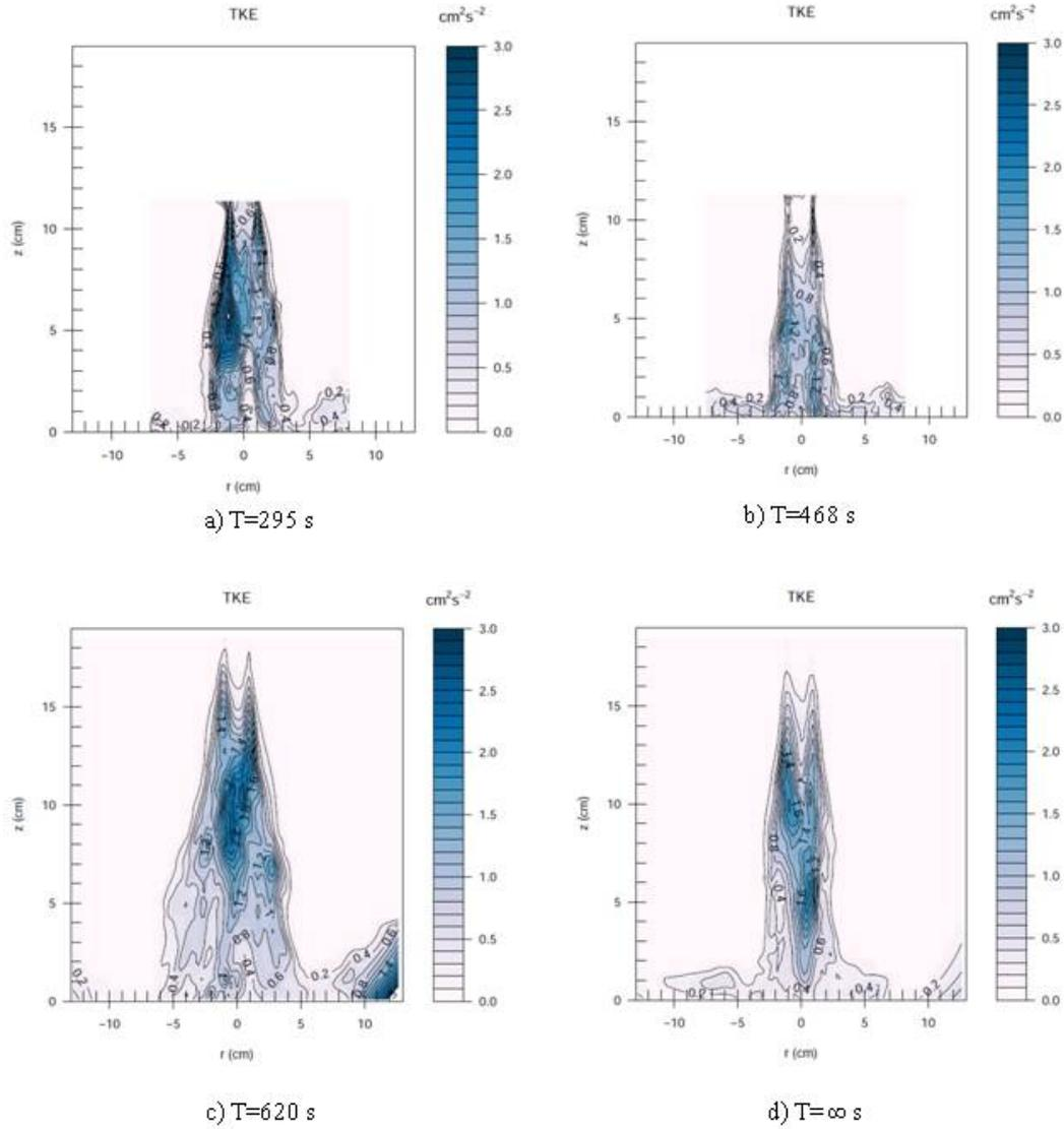
**Figure 4.** Turbulent kinetic energy for the four experiments.
