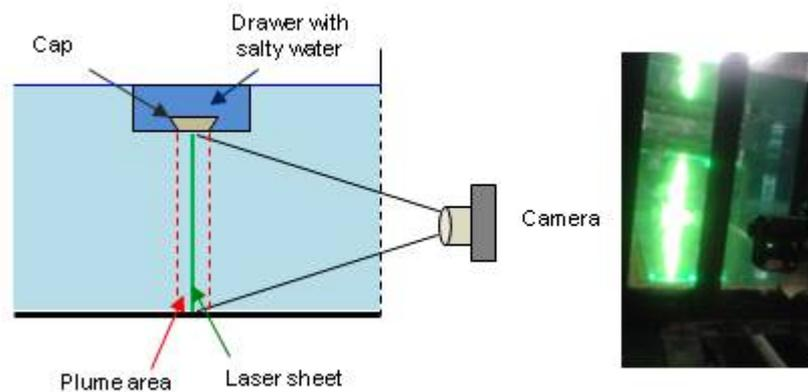
**Figure 1.** Left panel: a side view of the experimental setup. Right panel: an image of the plume produced during the data acquisition.
